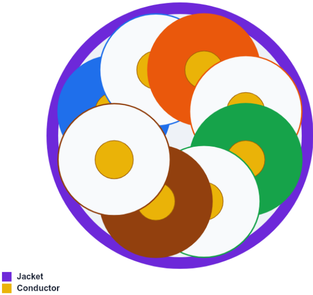
Cross-section diagram U/UTP — unshielded twisted pairs
