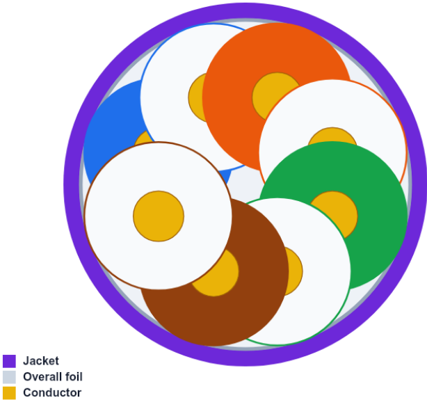
Cross-section diagram F/UTP — overall foil screen
