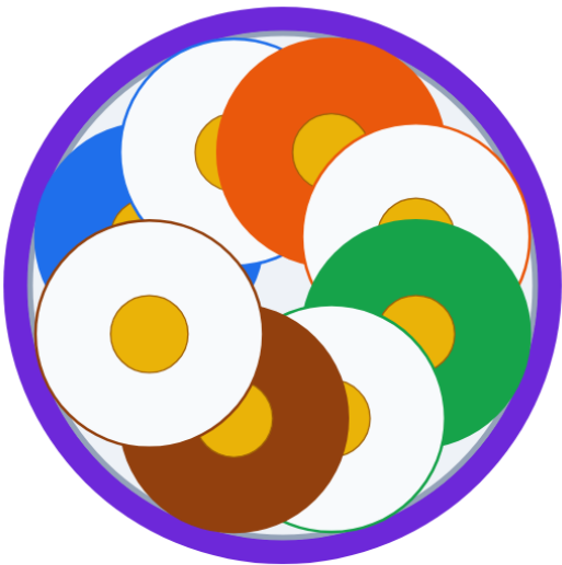
Cross-section diagram F/UTP — overall foil screen
