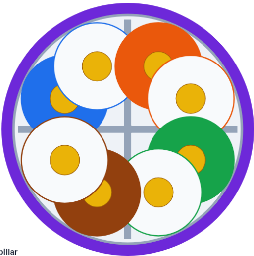
Cross-section diagram F/UTP — overall foil + cross pillar
